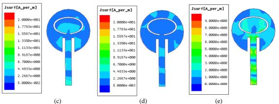
Fig. 3Simulated surface current distributions of the proposed penta-band antenna observed at (a) 2.33 GHz, (b) 3.44 GHz, (c) 8.13GHz, (d) 8.67 GHz and (e) 10.09 GHz
