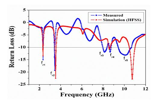
Fig. 2 Comparison of simulated and experimental return loss characteristics of proposed antenna
